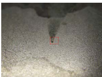
LOCAL ANODE CORROSION SAMPLE + 30MIN 3% NAACL SUBMERSION
